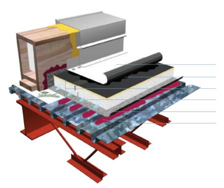
Lexcan Fleece-Backed membrane Lexcor Lexstick CA adhesive Fransyl Polybase R+ S Lexcor Adphalt adhesive **Lexcor Permate Stick SA Vapour Barrier** Lexcor Multigrip adhesive and primer
