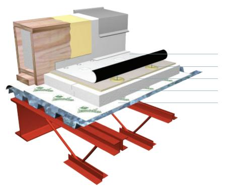
Lexcan White TPO HI-TUFF Membrane **Lexcor Lexgrip induction Screw and Plates Lexcor Lexboard Recover Board** Fransyl Izolon Insulation Lexcor Lexshield self-adhesive vapour barrier
