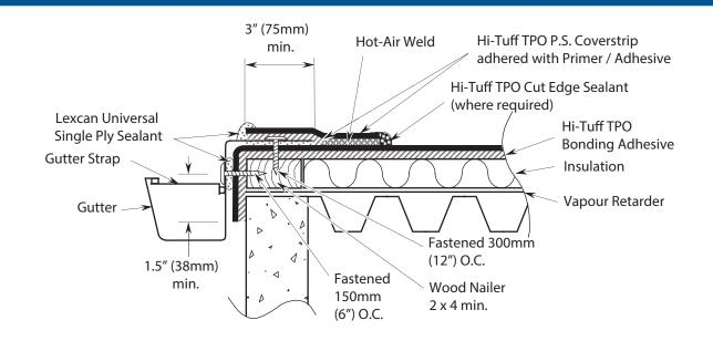
Comments: Gutter straps must be secured into fascia. Never installed on top of nailer.
