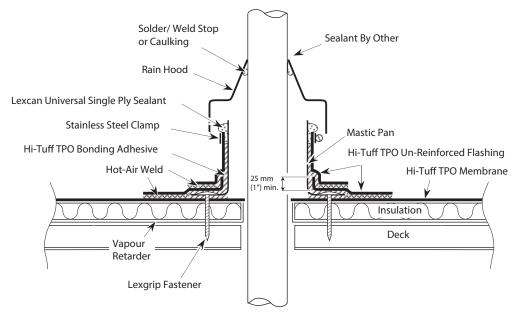
Comments: Rain Hood must be separated a minimum of 1 cm (1/2") from mastic pan to allow for condensation drainage.
