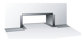
Bond Hi-Tuff TPO Un-Reinforced membrane piece to inside of scupper. Hot Air weld flaps that overlap Hi-Tuff TPO membrane.
