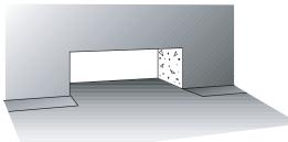
Step 1: Apply Hi-Tuff TPO membrane to deck & parapet
