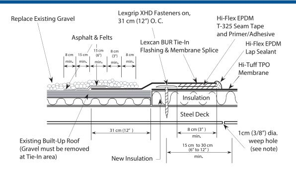
Note: When roof slope is toward new roofing system, drill a 1cm (3/8") diameter weep hole in the bottom flutes of the steel deck (rule not applicable for wood decks) along the perimeter of the tie-in 15cm (6" to 12") from the fastening plates.
