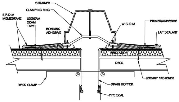
COMMENTS: I. EXTEND MEMBRANE 38 mm (1 1/2") BEYOND DRAIN BOLTS. PUNCTURE BOLT HOLES IN MEMBRANE. DO NOT CUT.
