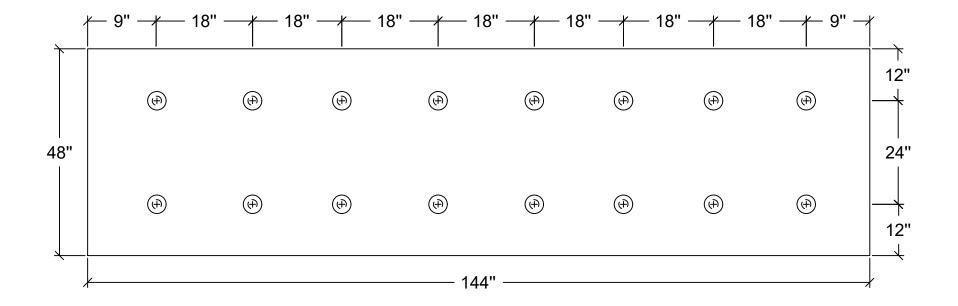
Induction welding attachments rates - Mach 12 System ROOFING SYSTEMS DETAIL
